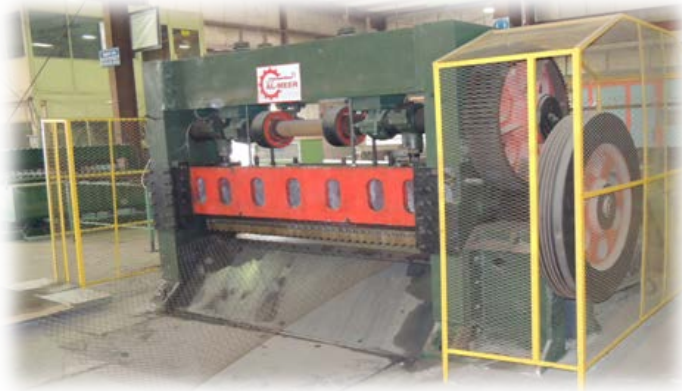
9. Expanded Metal Production Line
